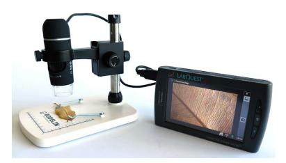
The magnification (small or large) and focus can be adjusted with a knob on the microscope body. The intensity of the LED light is adjusted by a knob on the microscope cable - if the source emits light itself (for example, pixels on the computer screen), switch the light off. On the other hand, it is recommended to have the light on when examining leaves, fabric, hairs and so on.
