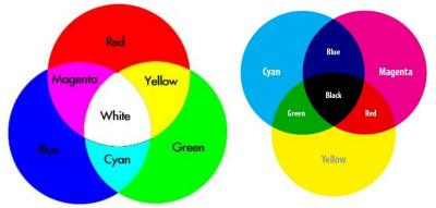
The difference is that whereas in the case of the display we add different colours to the resulting light (which is why it is sometimes called the *additive* colour mixing), pigments (printing inks, food dyes) act as colour filters, so this principle is also called the subtractive colour mixing. The pigments remove some parts of a light spectrum. So for example, the blue-green (cyan) dye absorbs everything except the blue and green colours, which are reflected.
