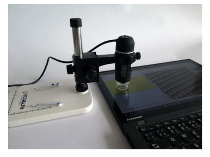
Launch the programme *Paint* in your computer and simultaneously display the application *Celestron MicroCapture Pro.* Use the "bucket" tool in *Paint* to make the whole area red. The microscope with large magnification reveals that only red subpixels are lit in the computer display.
