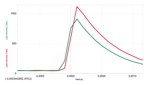
Simplified interpretation of this graph is that both light sensors captured the light at the same time. In this simplification the light travels any distance "immediately".
